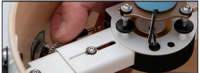
Insert cable plug (plug must snap into place)
