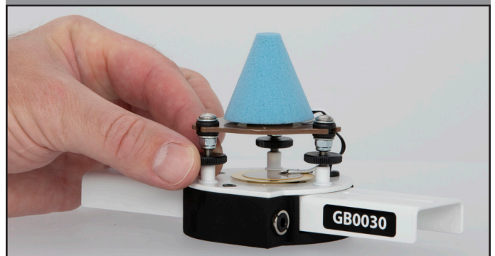
... the lock nuts have to be tightened again!
