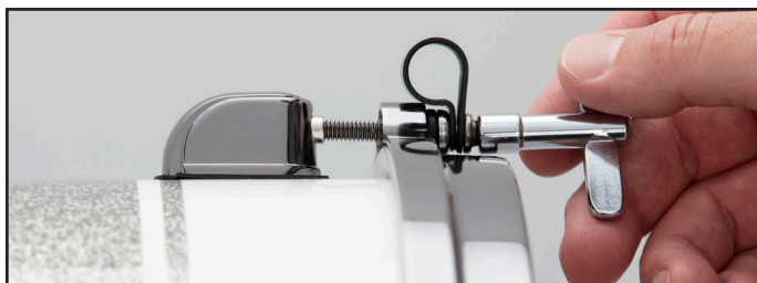
Tighten tuning screw with holder again
