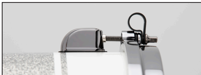
If bracket is too tight: Loosen tuning screw, Push bushing through, retighten tuning screw
