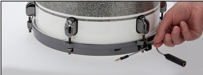
Pulling the cable through the socket holder
